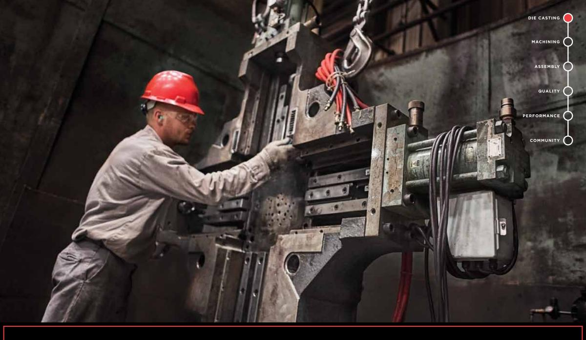
le CASTING: BEGINNING WITH THE BEST. Hot feed robotics pour molten aluminum into banks of massive die casting machines. Six-axis robots remove, cool, transport and deliver rock-solid covers, cylinder heads, and crankcases complete with cast-in iron liners that provide automotive-level durability. Making these core parts is a tough, complex interaction of technology, metallurgy, man and machine—but it's the surest way to lock world-class performance into every part.
